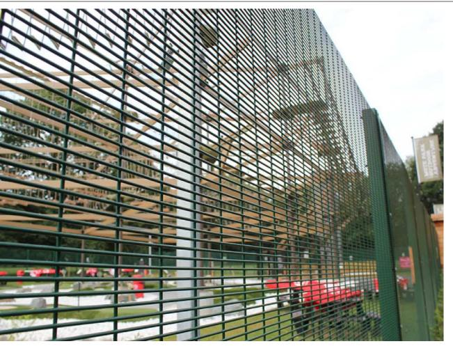
358 Welded Mesh Security Panels or similar equal and approved Restricted mesh width - 12.7 x 76.2mm x 4mm Posts - 80 x 60mm square section Height 1800mm Colour RAL - GREEN
